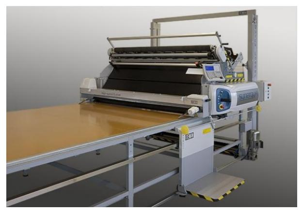
The SYNERGY line of cradle feed cloth spreading machines has been developed to allow ultra-fast bobbin change.
